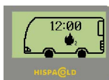
Preheater Screen running in programmed mode.
